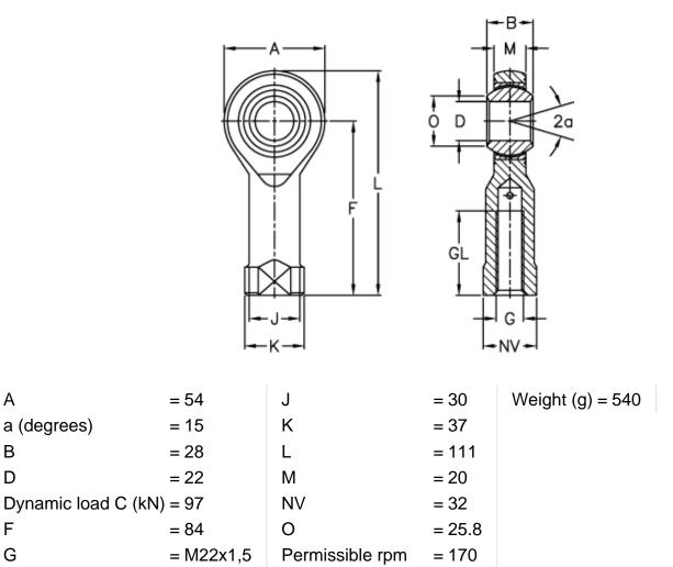
Static load C0 (kN) = 53
